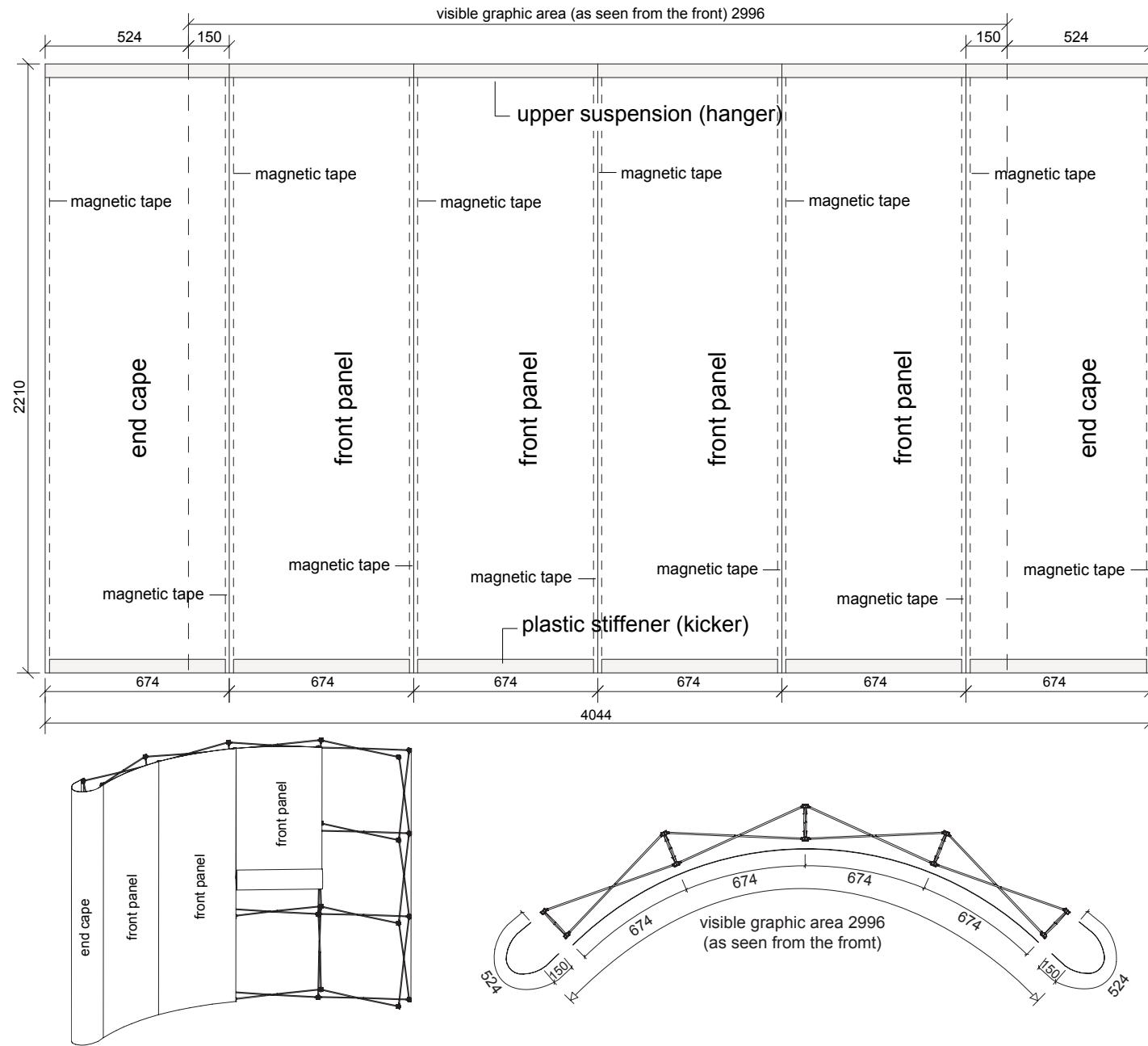
measurements in mm
