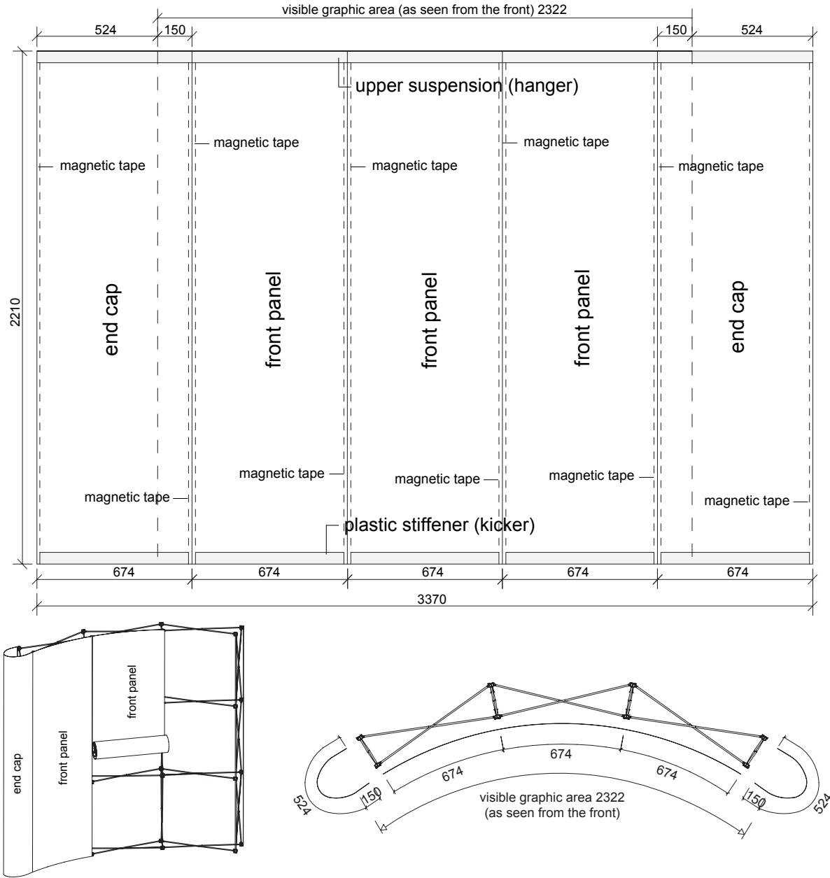
measurements in mm
